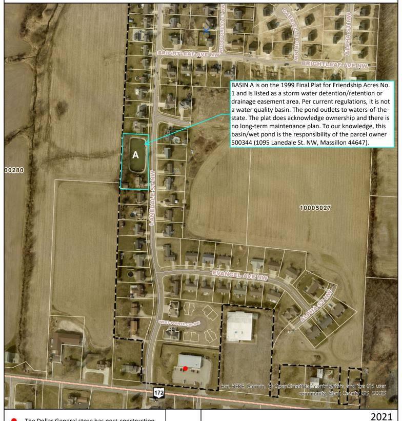
The Dollar General store has post-construction dry detention basin that is annual inspected. The basin is within a platted storm water detention area.
