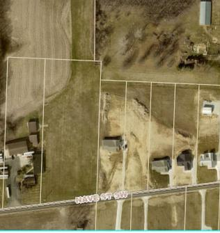
BASIN B is on the 1996 Dedication Plat and Roadway Improvements for University Drive and is listed as a storm water retention pond area. The pond outlets to waters-ofthe-state. The plat does not acknowledge ownership and there is no long-term maintenance plan on file. To our knowledge, this basin/wet pond is the responsibility of the parcel owner 10005774 (2550 University Dr SE, Massillon
