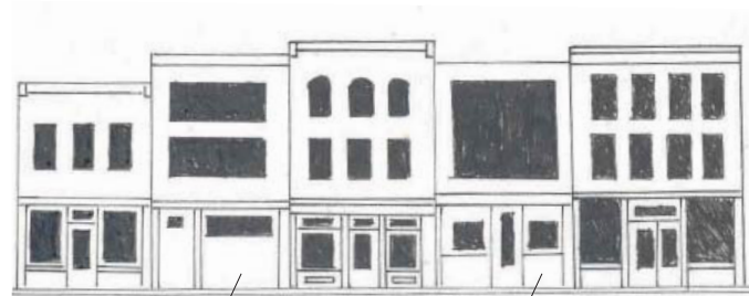
Inappropriate solid/void relationship to existing structures
